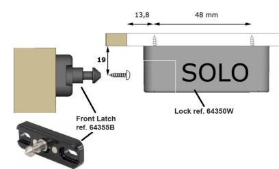
Installation with the latch **643 55B** This locking device is made of Zamak, a robust zinc aluminium alloy and the predetermined breaking point is 35 kg. The integrated pusher will automatically open light drawers and cabinet doors . The flexible pin allows tolerance of +/- 1 mm.
