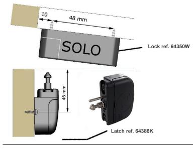
Installation with the latch **643 86K** Equipped with a mountin bracket and a spring, the latch gives a maximum confort during assembly based on the 3D adjustable fixing.
