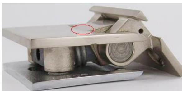
Photo of a REVERSI hinge forced beyond 90° opening.
